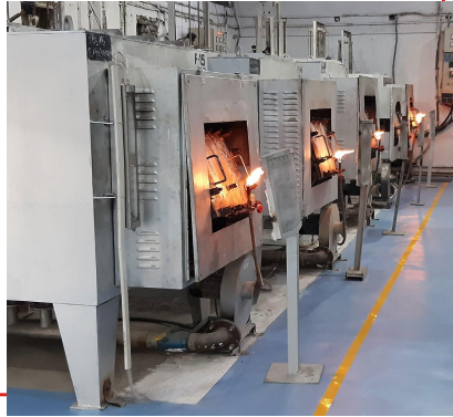
Annealing Services with Temperature mapping (TUS, SAT) as per AMS 2750 E
